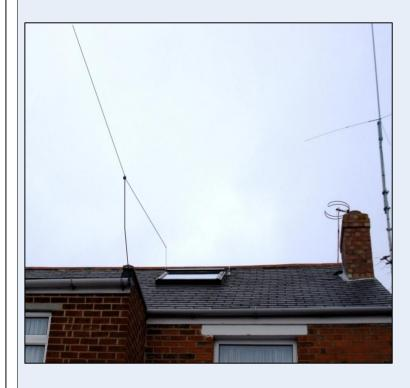
The K1POO antenna has the great advantage for me that the coax feed is very near the house, so it can hang down almost directly outside my window. My garden is only 16m long, so the antenna's shorter end is over the house's roof at 9.5m AGL and the longer end slopes down the garden to a washing line post and fibreglass pole with a combined height of 8.5m. The last 1.5m is bent down at 60 degrees at the end.
