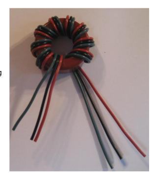
Next, trim, crimp together and solder <u>the left black wire</u> with the <u>right red wire</u> When the step is completed, it will look like the photo on the right:
