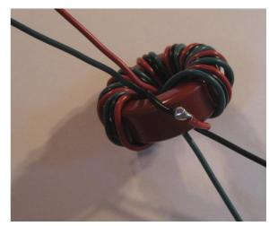
The next three steps should appear as shown in the right photo. Crimp and solder a #10 lug to the *left red* wire about 2" from the toroid. The completed lug will later connect to the antenna connection bolt on the top side of the enclosure.
