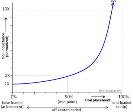
Required loading-coil inductance as function of coil placement
