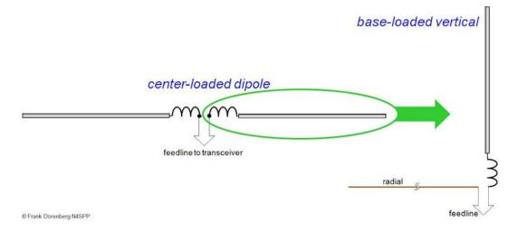
Discussions about loading of dipole antennas equally apply to vertical monopole antennas.
